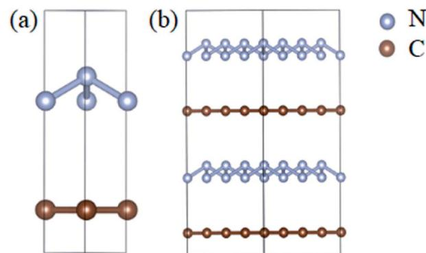
Fig. 1 The side view (left) for (a) the unit cell and (b) supercell ( $4 \times 4 \times 2$ ) of the A7@graphene crystal structure. The silver-gray and brown spheres are nitrogen atoms and carbon atoms, respectively.
