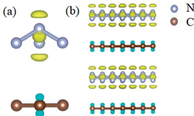
Fig. 4 The isosurface of electron density difference for (a) the unit cell and (b) supercell ( $4 \times 4 \times 2$ ) of the A7@graphene crystal structure. Blue and yellow denote the effective positive and negative charge respectively, while the panel is an isosurface of  $\pm 2.3 \times 10^{-4} (e \text{ \AA}^{-3})$ . The silver-gray and brown spheres are nitrogen atoms and carbon atoms, respectively.
