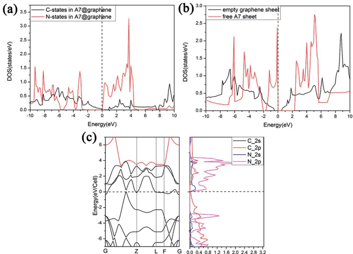
Fig. 6 Projected density of states (PDOS) for (a) the A7@graphene system, and (b) free polymeric nitrogen sheet and empty graphene sheet. (c) The band-decomposed charge-density of the A7@graphene system. A 0.05 eV broadening is used.
