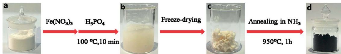
Scheme 1 Illustration of the typical N,P,Fe-NPC preparation. Photographs of Pueraria lobata powder (a), Pueraria lobata gel containing \text{H}_3\text{PO}_4 and \text{Fe}(\text{NO}_3)_3 \cdot 9\text{H}_2\text{O} (b), the material precursor obtained from the gel (c), and typical N,P,Fe-NPC (d).
