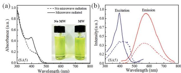
Fig. 1 (a) Normalized UV-vis absorption spectrum of 2%  $\text{Mn}^{2+}$ -doped CdSe QDs (SA5) with microwave radiation (solid line) and without microwave (MW) radiation (dashed line). Inset shows the photographs of CdSe QDs solution before and after MW treatment. (b) Photoluminescence excitation and emission spectrum of the same SA5 sample with microwave radiation (solid line) and without microwave radiation (dashed line) respectively.
