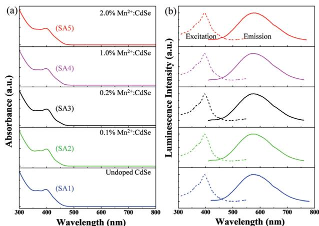
**Fig. 2** (a) Normalized UV-vis absorption and (b) PL excitation (dashed line) and emission (solid line) spectra of all five CdSe QDs sample with various Mn<sup>2+</sup>-dopant ion concentration synthesized in aqueous medium.
