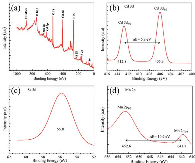
Fig. 4 (a) Survey X-ray photoelectron spectrum of 2%  $\text{Mn}^{2+}$ -doped CdSe QDs (SA5). (b) & (c) High-resolution spectrum of Cd 3d electrons showing doublet splitting with binding energy separated by 6.9 eV and Se 3d respectively. (d) High-resolution spectrum of Mn 2p core electrons showing doublet splitting with binding energy separated by 10.9 eV.
