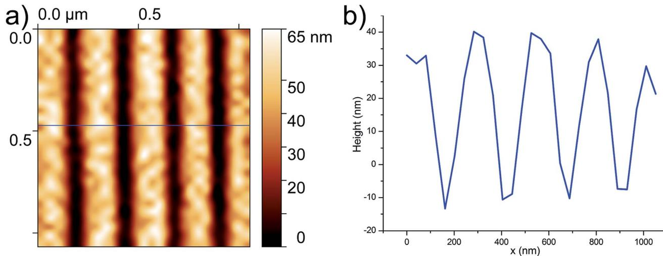
Fig. 3 AFM image (a) of a PMMA mask exposed to the ideal EBL dose of  $670 \mu\text{C cm}^{-2}$ , measured after development: the gold surface underneath the mask is exposed, yet the lines are still separate; a line profile taken on the blue line is reported in (b).
