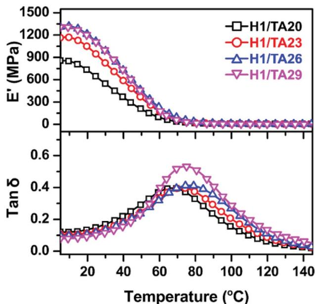
Fig. 3 DMA curves of the cured thermosets.
