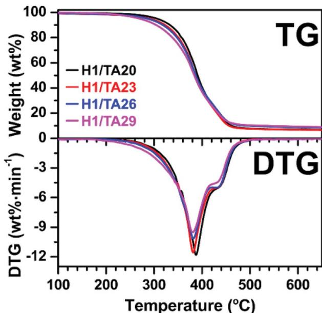
Fig. 4 TG (a) and DTG (b) curves of the cured thermostets under a  $N_2$  atmosphere.
