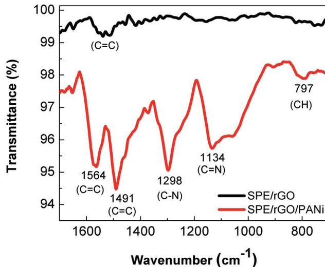
Fig. 3 ATR-FTIR spectra of rGO (black) and rGO-PANi (red) films. For rGO: 1400–1600  $\text{cm}^{-1}$  (C=C stretching), 1010  $\text{cm}^{-1}$  ( $-\text{C}-\text{O}-$ ). For rGO/PANi: 1564 and 1491  $\text{cm}^{-1}$  (C=C stretch), 1298  $\text{cm}^{-1}$  (C-N stretch), 1134  $\text{cm}^{-1}$  (C=N), 797  $\text{cm}^{-1}$  (C-H).
