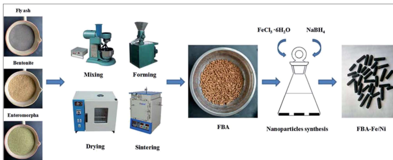
Fig. 1 Schematic diagram of FBA-Fe/Ni preparation.
