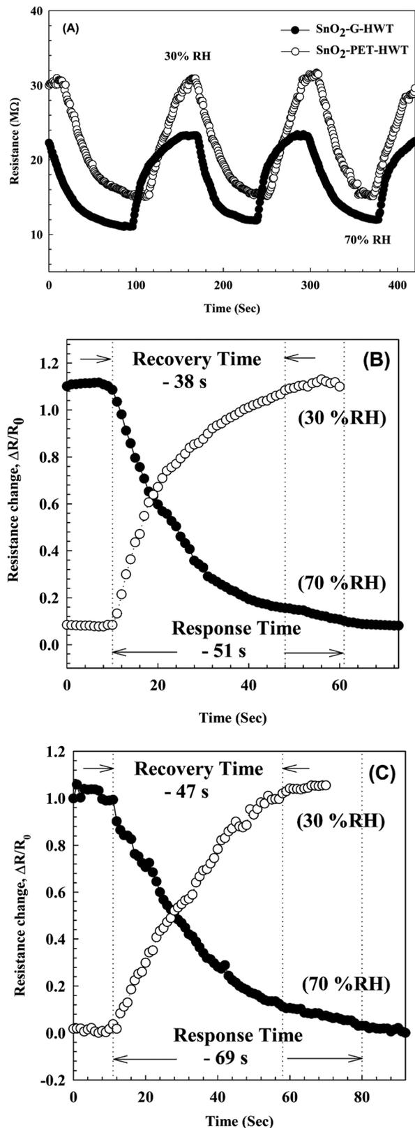
Fig. 10 (A) The resistance changes in the SnO<sub>2</sub>-G-HWT and SnO<sub>2</sub>-PET-HWT humidity sensor under three cycles of exposure to different % RH values from 30% to 70% at 20 ± 1 °C. (B) and (C) showed the humidity response (humidification from 30 to 70% RH) and recovery (desiccation from 70 to 30% RH) curves of SnO<sub>2</sub>-G-HWT and SnO<sub>2</sub>-PET-HWT humidity sensor at 20 ± 1 °C, respectively.
