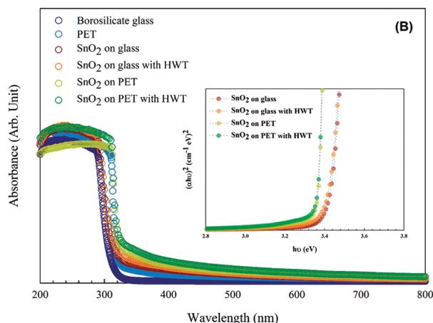
Fig. 3 The optical properties of the SnO<sub>2</sub> samples. (A) The transmittance results for SnO<sub>2</sub>. The inset photographs show (a) SnO<sub>2</sub>-G and (b) SnO<sub>2</sub>-PET samples after the HWT process. (B) The absorbance and band-gap spectra.
