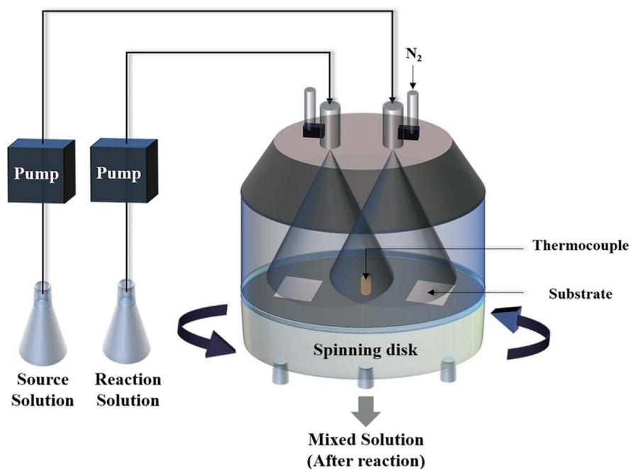
Fig. 1 A schematic diagram of the spin-spray apparatus.
