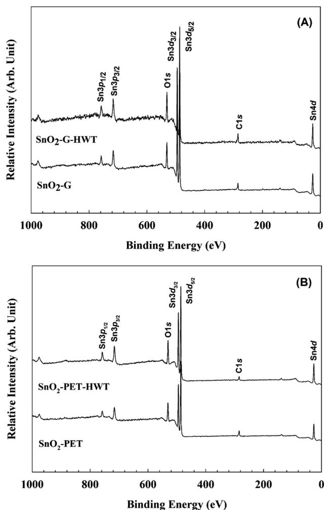
Fig. 5 The XPS survey spectrum of (A) SnO<sub>2</sub>-G and (B) SnO<sub>2</sub>-PET.
