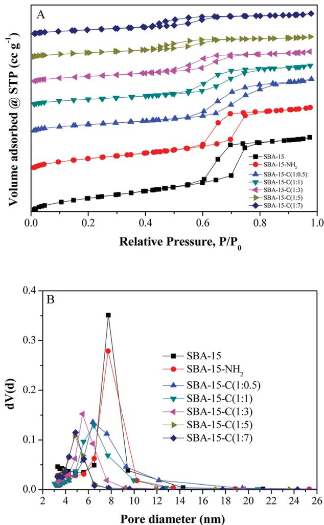
Fig. 4 Nitrogen adsorption/desorption isotherms and pore size distributions of SBA-15, SBA-15-NH<sub>2</sub> and SBA-15-C under different substrate proportions.
