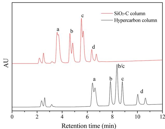
Fig. 7 The separation of oligosaccharide isomers on the SiO<sub>2</sub>-C (5 μm) and hypercarbon columns (150 mm × 4.6 mm): (a) LNDFH-II, (b) LNDFH-I, (c) LNFP-II, (d) LNFP-I; (a and b) and (c and d) were two pairs of isomers, and each compound corresponded to double peaks due to the effect of α/β anomeric splitting of saccharide.
