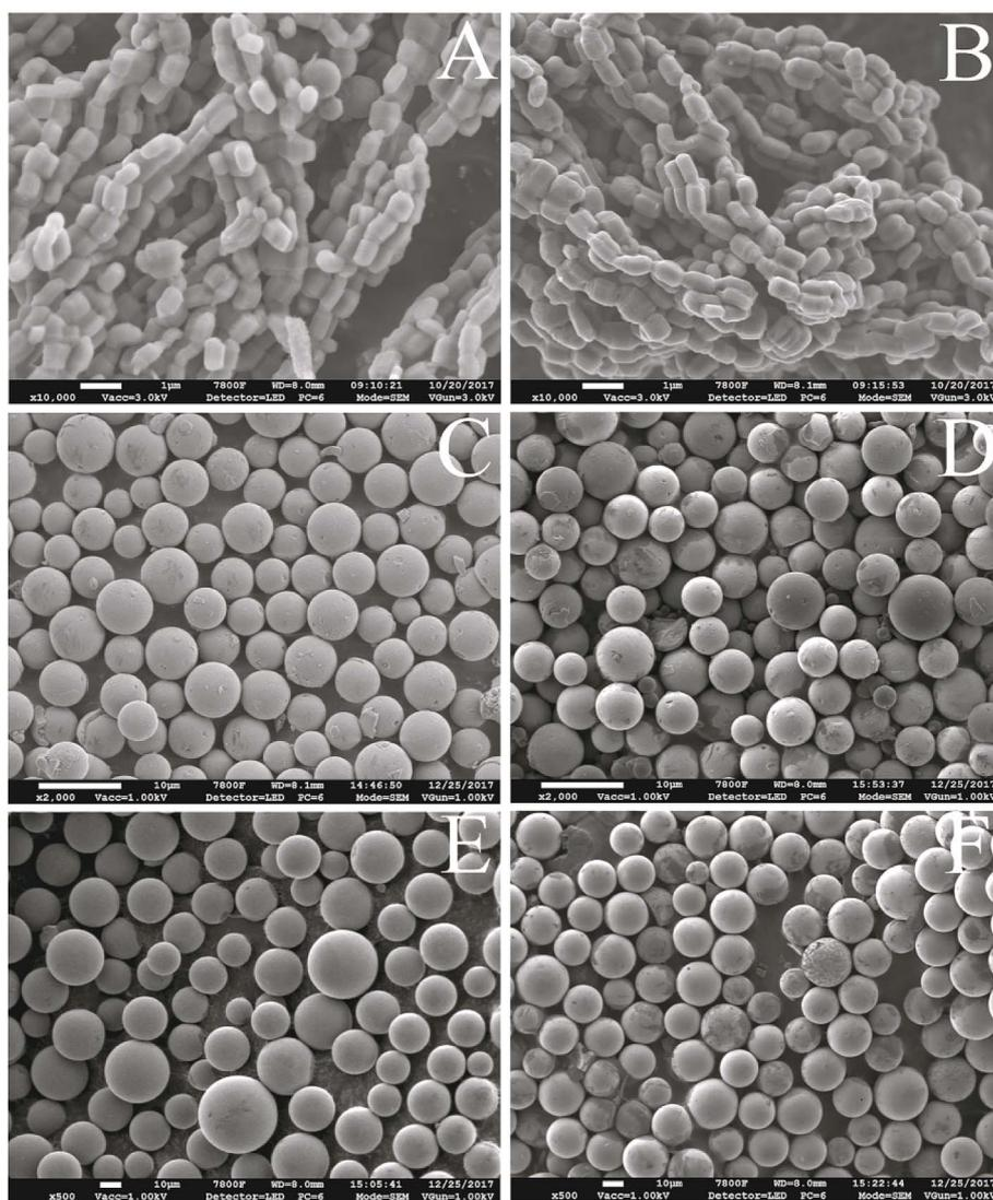
Fig. 2 SEM images of SBA-15 (A), SBA-15-C (B), SiO<sub>2</sub> (5 μm, C), SiO<sub>2</sub>-C (5 μm, D), SiO<sub>2</sub> (30 μm, E), and SiO<sub>2</sub>-C (30 μm, F), and the scale bars of (A and B) and (C–F) were 1 and 10 μm, respectively.
