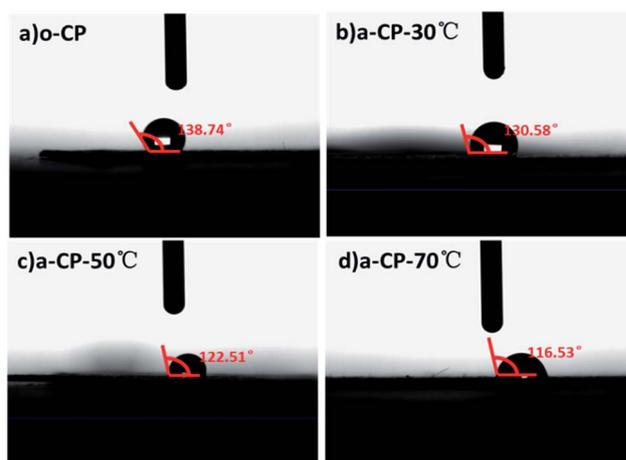
Fig. 3 The contact angles of different CPs.
