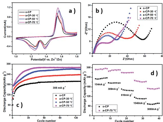
Fig. 4 CV curves of the  $\text{MnO}_2/\text{CP}$  electrode in 2 M  $\text{ZnSO}_4$  and 0.2 M  $\text{MnSO}_4$  hybrid aqueous electrolytes at a sweep rate of  $0.5 \text{ mV s}^{-1}$  (a), electrochemical impedance spectroscopy (EIS) after the CV test (b), and cyclic and rate performances of the cells utilizing different substrates (c and d).
