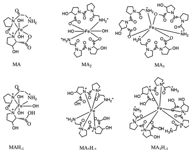
Fig. 3 The possible structures of  $[MA_nH_m]$ . M indicates the Fe(III) ion, A indicates the ligand Gly-Pro-Hyp.
