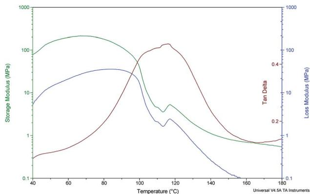
Fig. 2 DMA analysis for Nafion 117 “as received and oriented”. The brown line refers to  $\tan \delta$ , the green line refers to the storage modulus ( $\log E'$ ) and the blue line refers to the loss modulus ( $\log E''$ ). Sample parameters: length 8.95 mm, width 6.62 mm, thickness 0.18 mm.
