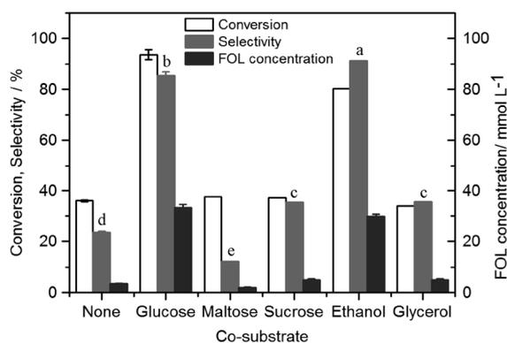
Fig. 3 Effect of co-substrate on reduction of furfural by whole cell catalytic of *B. coagulans* NL01. Conditions: 42 mM FAL, 10 g L<sup>-1</sup> co-substrate, 9 mg (dry weight) per mL microbial cells, 25 mL phosphate buffer (200 mM pH 7.0), 150 rpm, 50 °C; anaerobic reaction for 24 h under the above conditions, with different letters representing significant differences between the treatment means ( $p < 0.05$ ).
