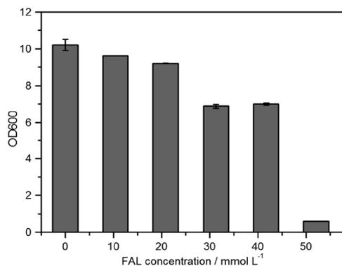
Fig. 1 Effect of FAL concentration on cell viability. Cell viability was measured by turbidity measurements at 600 nm (OD<sub>600</sub>) after 60 h fermentation.
