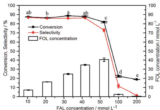
Fig. 4 Effect of substrate concentration on reduction of furfural by whole cell catalytic of *B. coagulans* NL01. Conditions: 0–200 mM FAL, 10 g L<sup>-1</sup> glucose, 9 mg (dry weight) per mL microbial cells, 25 mL phosphate buffer (200 mM pH 7.0), 150 rpm, 50 °C; anaerobic reaction for 24 h under the above conditions, with different letters representing significant differences between the treatment means ( $p < 0.05$ ).
