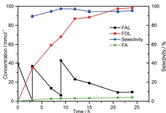
Fig. 9 FOL production in a fed-batch culture of *B. coagulans* NL01. Conditions: 40 mM FAL, 20 g L<sup>-1</sup> glucose, 9 mg (dry weight) per mL microbial cells, 25 mL phosphate buffer (200 mM pH 7.0), 150 rpm, 50 °C. After FAL was almost used up, 0.925 mmol FAL were supplemented.
