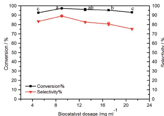
Fig. 6 Effect of cell concentration on reduction of furfural by whole cell catalytic of *B. coagulans* NL01. Conditions: 42 mM FAL, 20 g L<sup>-1</sup> glucose, 5–21 mg (dry weight) per mL microbial cells, 25 mL phosphate buffer (200 mM pH 7.0), 150 rpm, 50 °C; anaerobic reaction for 24 h under the above conditions, with different letters representing significant differences between the treatment means ( $p < 0.05$ ).
