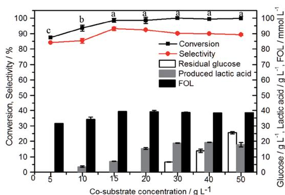
Fig. 5 Effect of co-substrate concentration on reduction of furfural by whole cell catalytic of *B. coagulans* NL01. Conditions: 42 mM FAL, 5–50 g L<sup>-1</sup> glucose, 9 mg (dry weight) per mL microbial cells, 25 mL phosphate buffer (200 mM pH 7.0), 150 rpm, 50 °C; anaerobic reaction for 24 h under the above conditions, with different letters representing significant differences between the treatment means ( $p < 0.05$ ).
