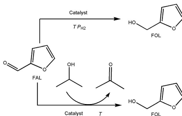
**Scheme 1** Chemical conversion of FAL into FOL (catalysts represent noble metal and non-noble metals;  $T = 130\text{--}200\text{ }^\circ\text{C}$ ; high H<sub>2</sub> pressure about 2.0 MPa).
