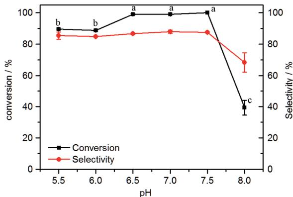
Fig. 7 Effect of pH on reduction of furfural by whole cell catalytic of *B. coagulans* NL01. Conditions: 42 mM FAL, 20 g L<sup>-1</sup> glucose, 9 mg (dry weight) per mL microbial cells, 25 mL phosphate buffer (200 mM pH 5.5–8.0), 150 rpm, 50 °C; anaerobic reaction for 24 h under the above conditions, with different letters representing significant differences between the treatment means ( $p < 0.05$ ).
