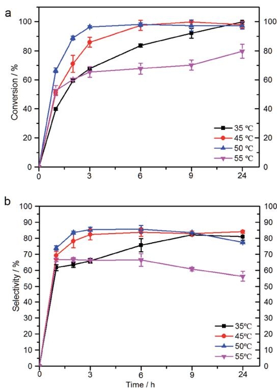
Fig. 8 Effect of temperature on reduction of furfural by whole cell catalytic of *B. coagulans* NL01. (a) The conversion of FAL; (b) the selectivity of FOL. Conditions: 42 mM FAL, 20 g L<sup>-1</sup> glucose, 9 mg (dry weight) per mL microbial cells, 25 mL phosphate buffer (200 mM pH 7.0), 150 rpm, 35–55 °C; anaerobic reaction for 24 h under the above conditions.
