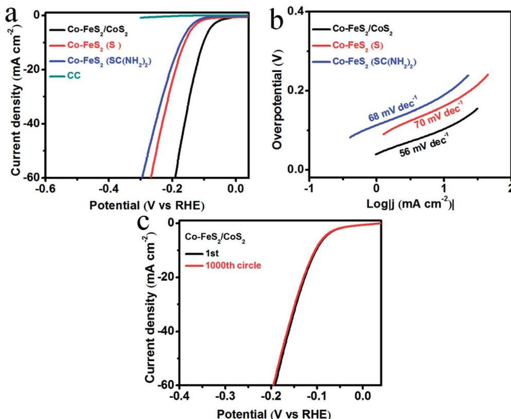
Fig. 4 (a) LSV curves of Co-FeS<sub>2</sub>/CoS<sub>2</sub>, Co-FeS<sub>2</sub>/CoS<sub>2</sub> (S), Co-FeS<sub>2</sub> (SC(NH<sub>2</sub>)<sub>2</sub>), and bare CC for HER in  $0.5 \text{ M H}_2\text{SO}_4$  solution; (b) corresponding Tafel plots; (c) LSV curves of Co-FeS<sub>2</sub>/CoS<sub>2</sub> before and after 1000 cycles.
