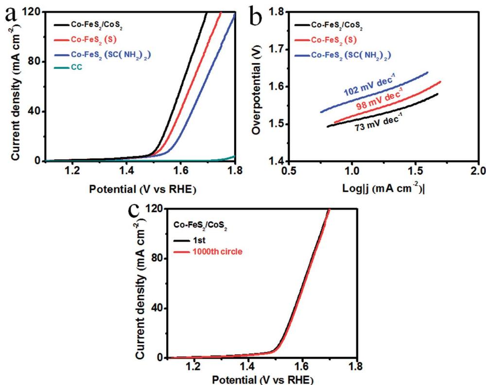
Fig. 3 (a) LSV curves of Co-FeS<sub>2</sub>/CoS<sub>2</sub>, Co-FeS<sub>2</sub> (S), Co-FeS<sub>2</sub> (SC(NH<sub>2</sub>)<sub>2</sub>), and bare CC for OER in 1 M KOH solution; (b) corresponding Tafel plots; (c) LSV curves of Co-FeS<sub>2</sub>/CoS<sub>2</sub> before and after 1000 CV cycles.
