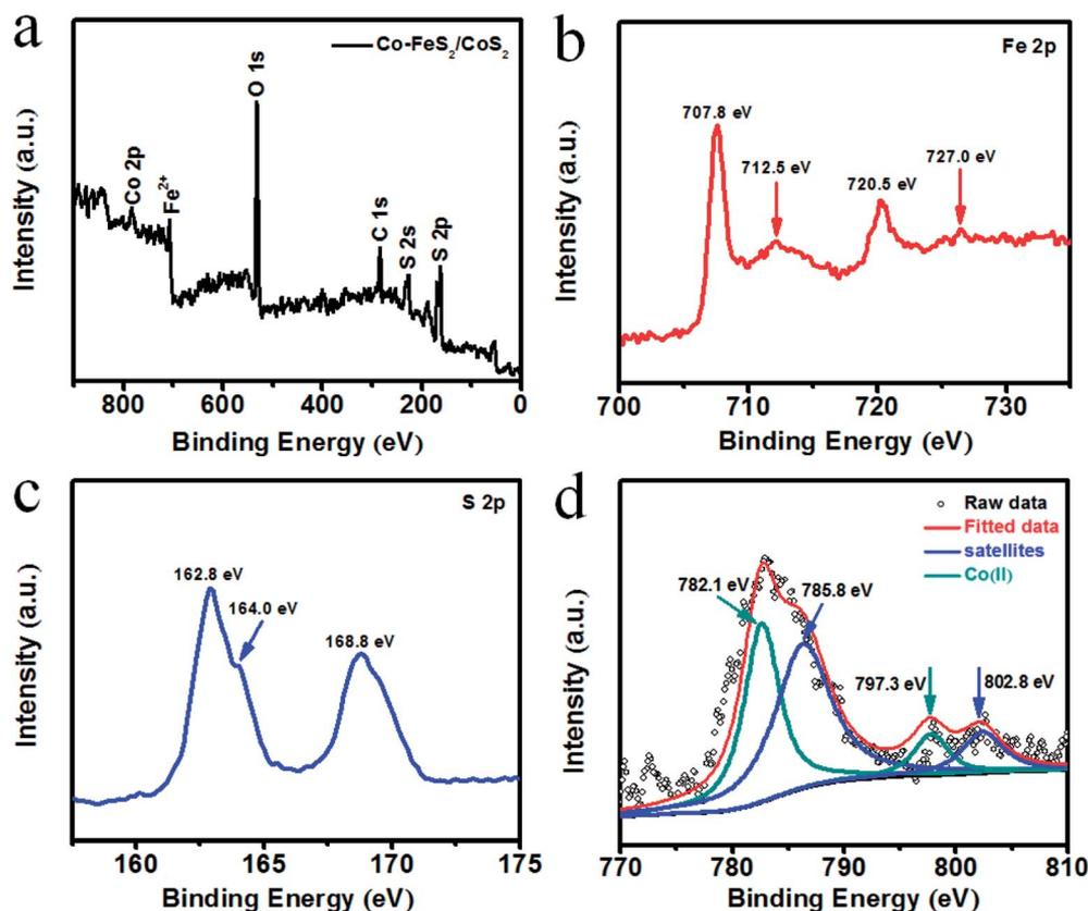
Fig. 2 (a) XPS survey spectrum for Co-FeS<sub>2</sub>/CoS<sub>2</sub>; XPS spectra of the Co-FeS<sub>2</sub>/CoS<sub>2</sub> from (b) Fe 2p, (c) S 2p, (d) Co 2p.
