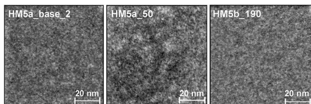
Fig. 6 HAADF-STEM images of the HM prepared by the STP of **4a** and **1** with the use of a base catalyst (HM5a\_base\_2, DABCO, 9.0 mol%/1 wt%, 120 °C, 2 h), the HM prepared by thermally induced STP of **4a** and **1** (HM5a\_50, equimolar, 170 °C, 2 h) and the HM prepared by thermally induced STP of **4b** and **1** (HM5b\_190, equimolar, 190 °C, 2 h).
