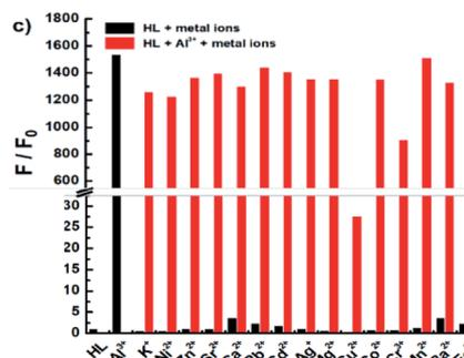
Fig. 5 (a) Fluorescence emission spectral changes of HL induced by various metal ions (5.0 equivalents) in acetonitrile ( $2.0 \times 10^{-5} \text{ mol L}^{-1}$ ) by excitation at 420 nm; (b) photos of fluorescence changes in acetonitrile; (c) the fluorescence intensity at 521 nm of HL upon addition of various metal ions (black bars: HL with metal ions; red bars: HL with other metal ions and  $\text{Al}^{3+}$ ) in acetonitrile.
