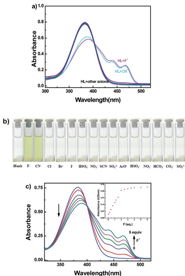
Fig. 6 (a) Absorption spectral change of HL induced by various metal ions (5.0 equiv.) in acetonitrile ( $2.0 \times 10^{-5} \text{ mol L}^{-1}$ ); (b) photos of color changes in acetonitrile; (c) absorption spectra and color of HL induced by F<sup>-</sup> in acetonitrile ( $2.0 \times 10^{-5} \text{ mol L}^{-1}$ ).
