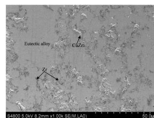
Fig. 2 The microstructure of the filler metal.
