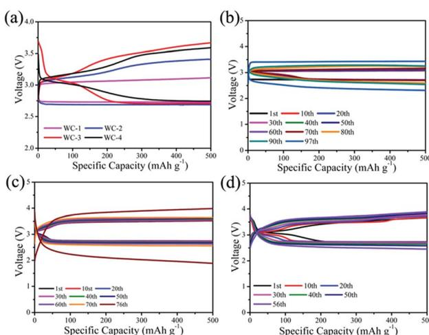
Fig. 7 Electrochemical performances of Li- $\text{O}_2$  cells with different cathode electrodes. Full discharge-charge capacity profiles of Li- $\text{O}_2$  cells with WC-1, WC-2, WC-3 and WC-4 at  $100 \text{ mA g}^{-1}$  (a). Charge-discharge curves of Li- $\text{O}_2$  cells under fixed capacity of  $500 \text{ mA h g}^{-1}$  at  $100 \text{ mA g}^{-1}$  and different cycles: (b) with WC-1 and LiI, (c) with WC-2 and LiI, (d) with WC-3 and LiI.
