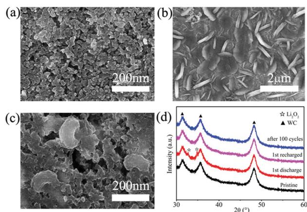
Fig. 5 SEM images of WC-1 cathode electrode at the pristine (a), after first discharge (b), and Li<sub>2</sub>O<sub>2</sub> morphology in cathode electrode after first discharge (c). (d) XRD patterns of cathode electrode at different charge–discharge status.
