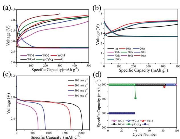
Fig. 4 (a) Full discharge–charge capacity profiles of Li–O<sub>2</sub> cells with WC-1, WC-2, WC-3, WC-4, g-C<sub>3</sub>N<sub>4</sub> and C at current density 100 mA g<sup>-1</sup>. (b) Cycles of Li–O<sub>2</sub> cells with WC-1 under fixed capacity of 500 mA h g<sup>-1</sup> at current density 100 mA g<sup>-1</sup>. (c) WC-1 cathodes at different current densities. (d) The cycling performances of the six cells with WC, g-C<sub>3</sub>N<sub>4</sub>, and C.
