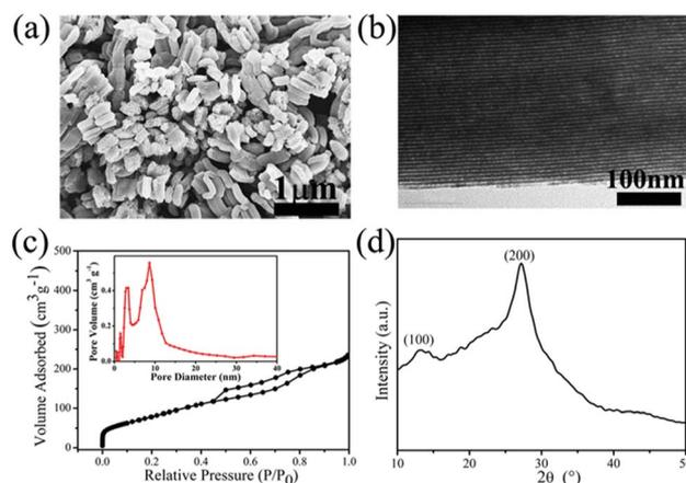
Fig. 1 Structural characterization of g-C<sub>3</sub>N<sub>4</sub>-1. (a) FE-SEM image of g-C<sub>3</sub>N<sub>4</sub>-1, (b) TEM image of g-C<sub>3</sub>N<sub>4</sub>-1, (c) nitrogen adsorption–desorption isotherms and pore size distribution of g-C<sub>3</sub>N<sub>4</sub>-1, (d) XRD patterns of g-C<sub>3</sub>N<sub>4</sub>-1.
