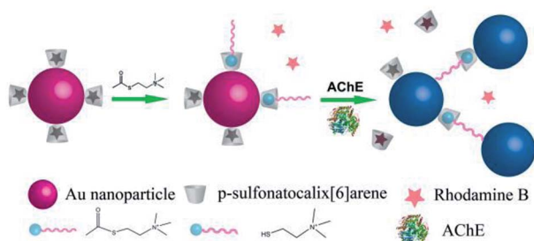
Fig. 1 System for detection of AChE activity based on RhB- p -SC 6 A-AuNPs aggregation and RhB release induced by the competitive host-guest interaction between p -SC 6 A-AuNPs and RhB/quaternary ammonium group.
