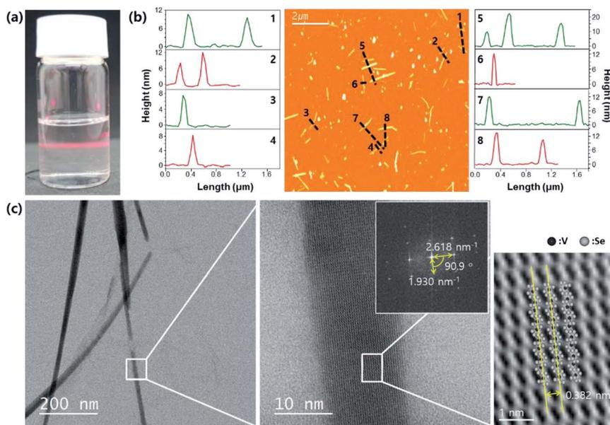
Fig. 4 Dispersion of  $V_2Se_9$  in IPA. (a) Tyndall effect of  $V_2Se_9$  dispersed solution. (b) AFM image of  $V_2Se_9$  chains deposited on Si/SiO<sub>2</sub> substrate and the height profiles along each dashed line. (c) TEM images and FFT pattern (inset) of dispersed  $V_2Se_9$  chains (the distance between two chains marked by yellow line is 0.382 nm).
