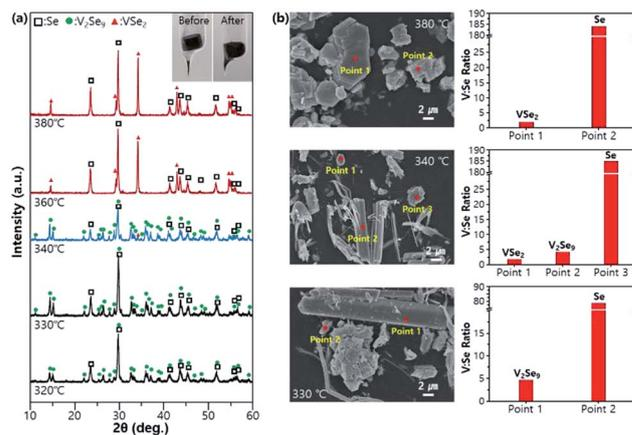
Fig. 2 (a) XRD patterns (inset is the optical images of sample before and after reaction) and (b) SEM images (left) and EDS analysis (right) of as-synthesized samples with  $T$  ranging from 320 °C to 380 °C. (V : Se ratio is 2 : 12.6).
