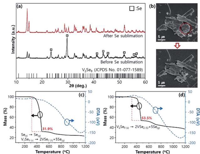
Fig. 3 Physical and chemical changes of  $V_2Se_9$  synthesized at 330 °C after Se sublimation. (a) XRD patterns (bottom: before Se sublimation, top: after Se sublimation), (b) SEM images (top: before Se sublimation, bottom: after Se sublimation, red dashed circle is Se) and (c and d) TG/DTA analysis in  $N_2$  atmosphere (left: before Se sublimation, right: after Se sublimation, red dashed line is Se sublimation and  $V_2Se_9$  decomposition step).
