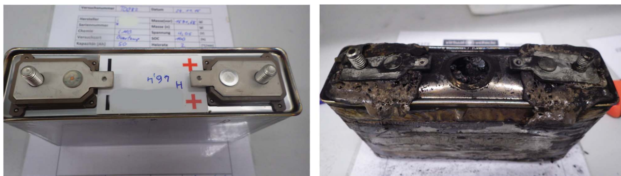
Fig. 2 Tested cell before and after the thermal runaway experiment. On the fresh cell, the burst-plate of the cell is hidden below the white sticker. After a thermal runaway the cell is heavily damaged: the burst plate is open, the plastic insulation of the terminals is melted and the cell casing is deformed by the pressure inside the cell.
