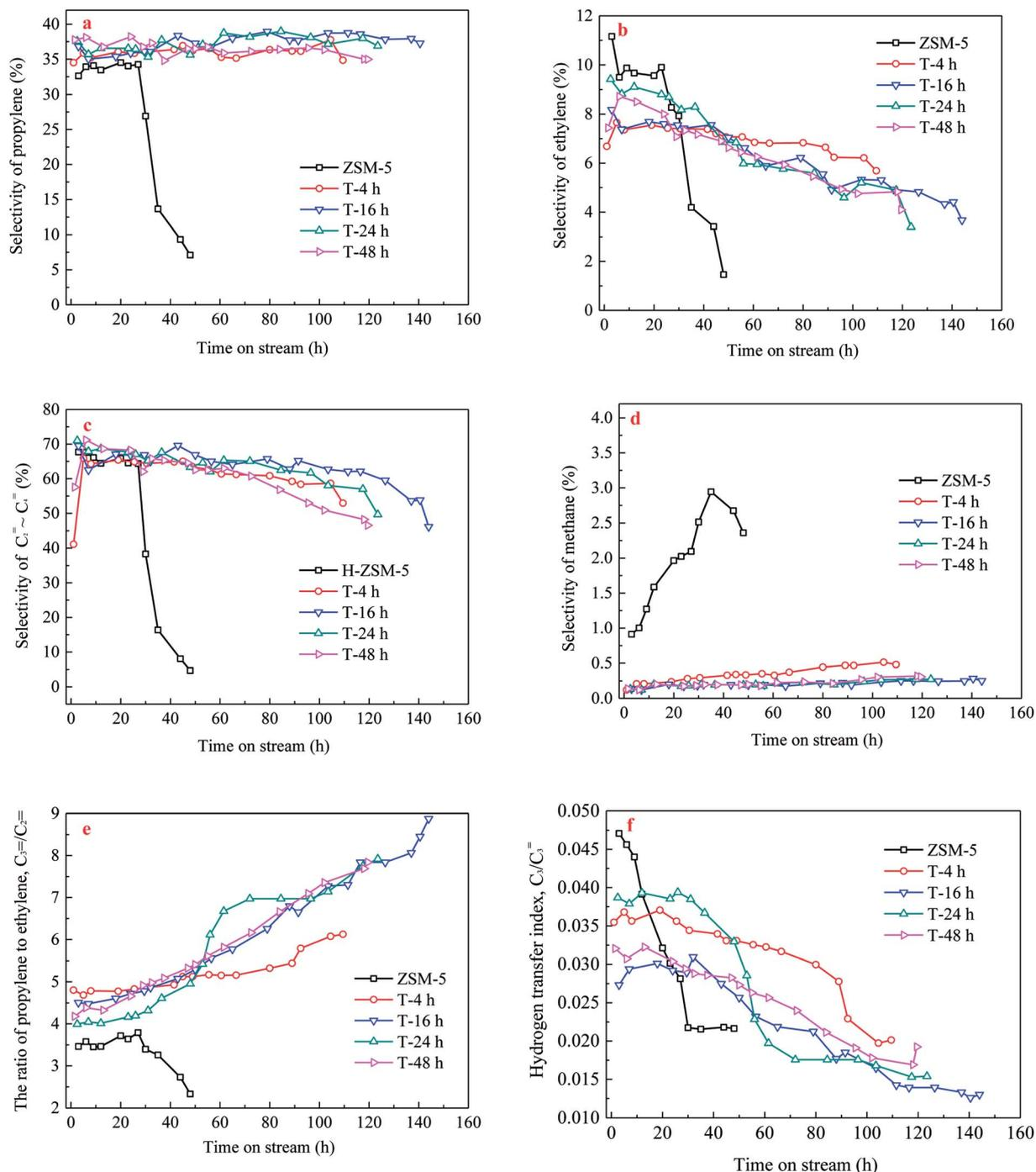
Fig. 9 Product selectivity ((a) propylene, (b) ethylene, (c)  $C_2 \sim C_4$ , (d) methane),  $C_3/C_2$  (e) and  $C_3$  hydrogen transfer index (f) of the parent and TEAOH-treated H-ZSM-5 samples for MTP reaction as a function of time. Reaction conditions:  $T = 480^\circ\text{C}$ ,  $\text{WHSV} = 4.5\text{ h}^{-1}$ ,  $P = 0.1\text{ MP}$ ,  $m(\text{H}_2\text{O}) : m(\text{CH}_3\text{OH}) = 1 : 1$ .
