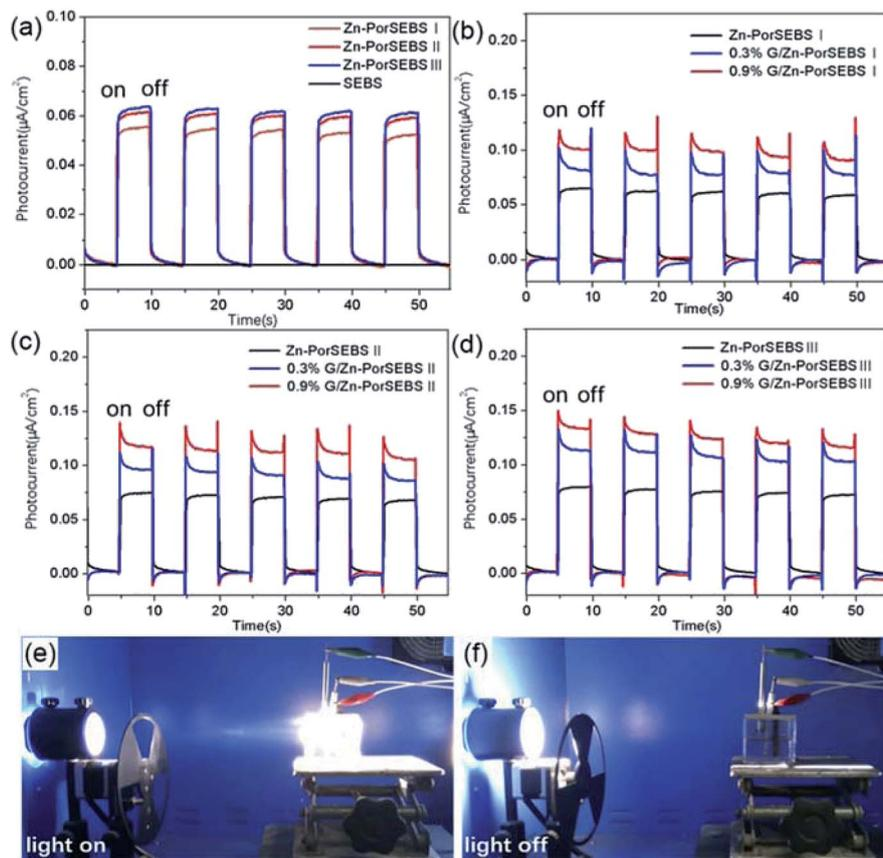
Fig. 4 Photocurrent switching response at 5 s intervals in a 0.3 V 1 M NaOH aqueous solution under 500 W Xenon lamp illumination. (a) Photocurrent response of neat SEBS and Zn-PorSEBS elastomer with different porphyrin grafting ratio. (b–d) Photocurrent response of Zn-PorSEBS elastomer and G/Zn-PorSEBS with different graphene content at the same porphyrin grafting ratio. (e and f) Photographs giving the light on/light off process.
