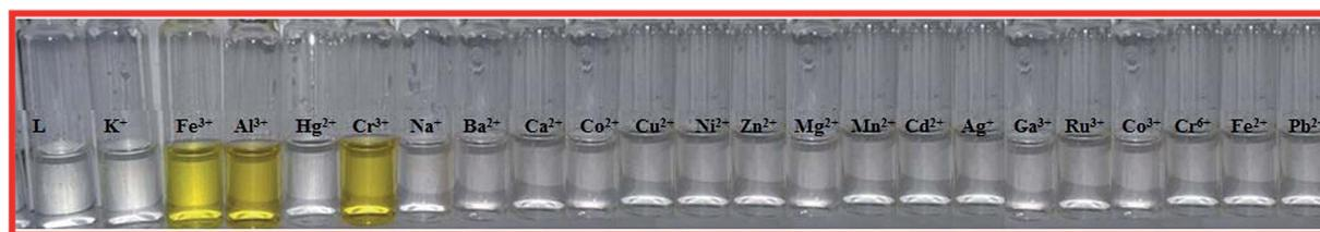
Fig. 3 The colour changes of L (10  $\mu\text{M}$ ) upon addition of various metal ions (1 equiv.) in  $\text{CH}_3\text{CN}-\text{H}_2\text{O}$  (1 : 1, v/v) at room temperature.
