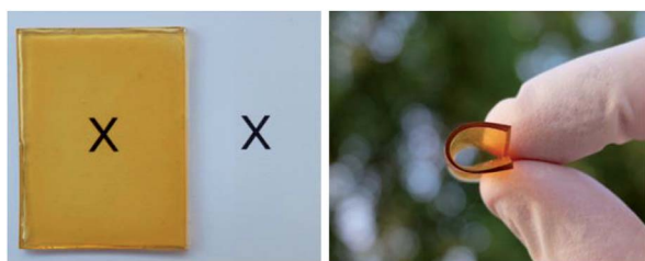
Fig. 8 Transparent and flexible EGS150 film.
