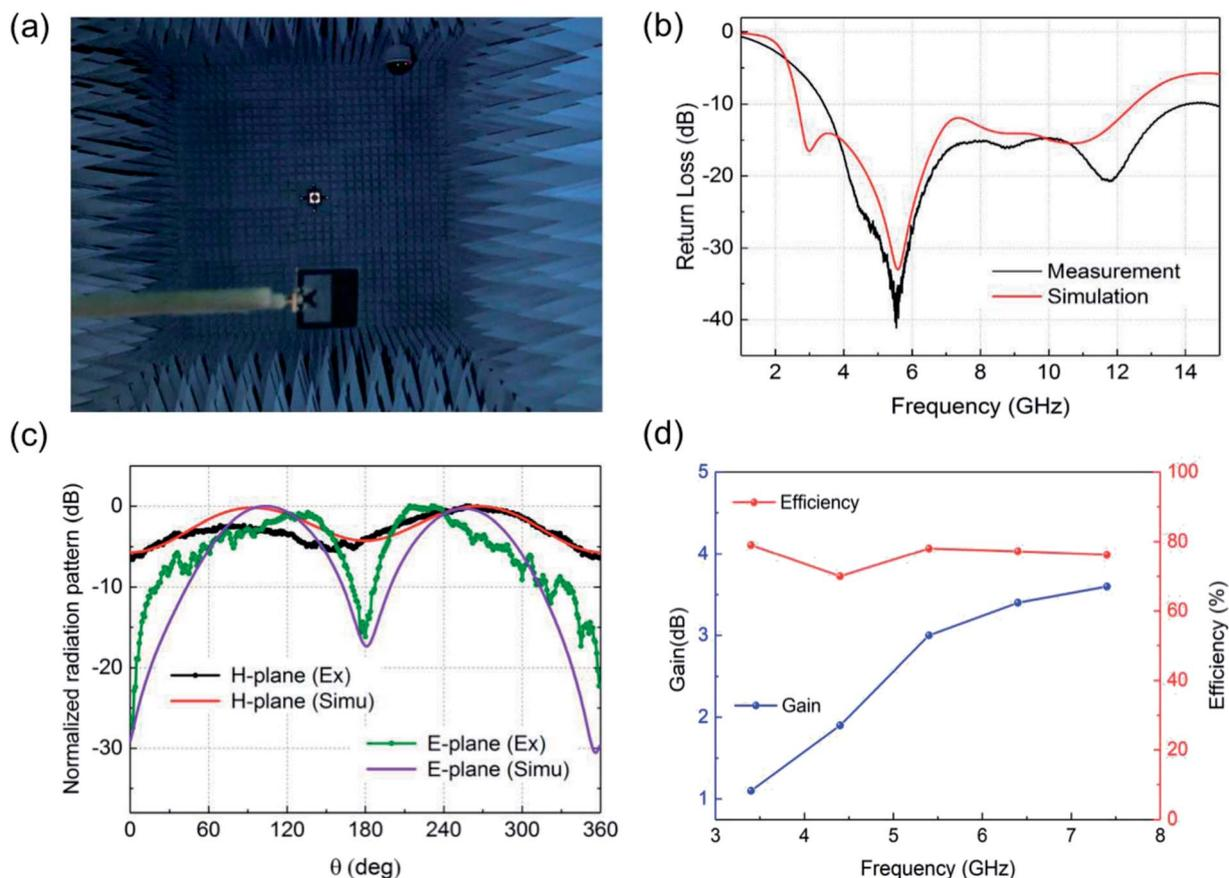
Fig. 4 (a) Image of radiation pattern measurements in anechoic chamber. (b) Simulated and measured return losses  $|S_{11}|$  of the slot antenna with beveled rectangular patch and two semicircle slots in the ground plane, and (c) the normalized radiation pattern in both E-(xz) and H-(yz) planes. (d) Measured gain and efficiency of the antenna as a function of frequency.
