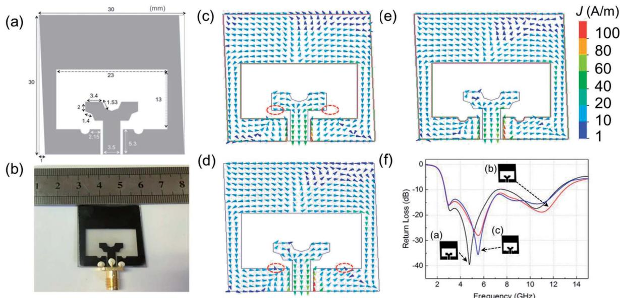
Fig. 3 Geometry (a) and photo (b) of the proposed slot antenna (unit: millimeters). (c) Surface current distributions at 5 GHz of three designed UWB slot antennas with simple Y shaped patch, (d) beveled Y shaped patch, and (e) beveled rectangular patch and two semicircle slots in the ground plane; (f) simulated return losses  $|S_{11}|$  of these three designed antennas.
