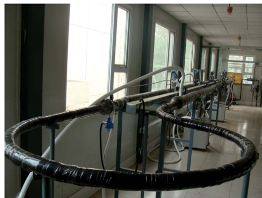
Fig. 1 The picture of high pressure hydrate experimental loop.
