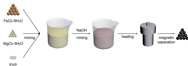
Fig. 1 Schematic illustration of the synthesis process of \text{MgFe}_2\text{O}_4 nanoparticles.
