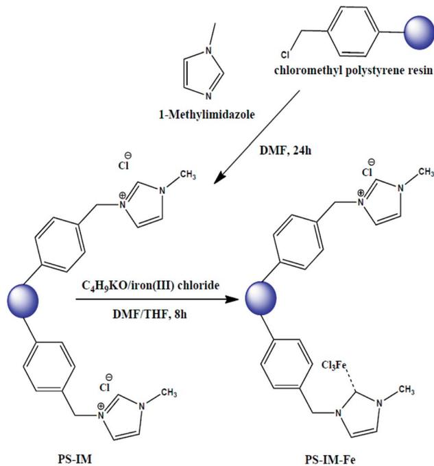
Fig. 1 Schematic diagram of synthesis of PS-Im and PS-Im-FeCl<sub>3</sub> catalyst.
