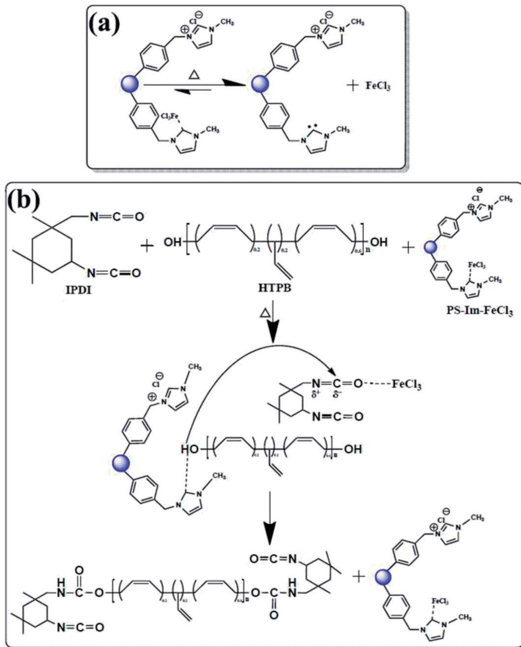
Fig. 6 (a) Reaction process of the PS-Im-FeCl<sub>3</sub> catalyst under applied heat and (b) catalytic activity mechanism. Dual activation of both polyol and isocyanate functional groups by the dissociated PS-Im-FeCl<sub>3</sub> catalyst.
