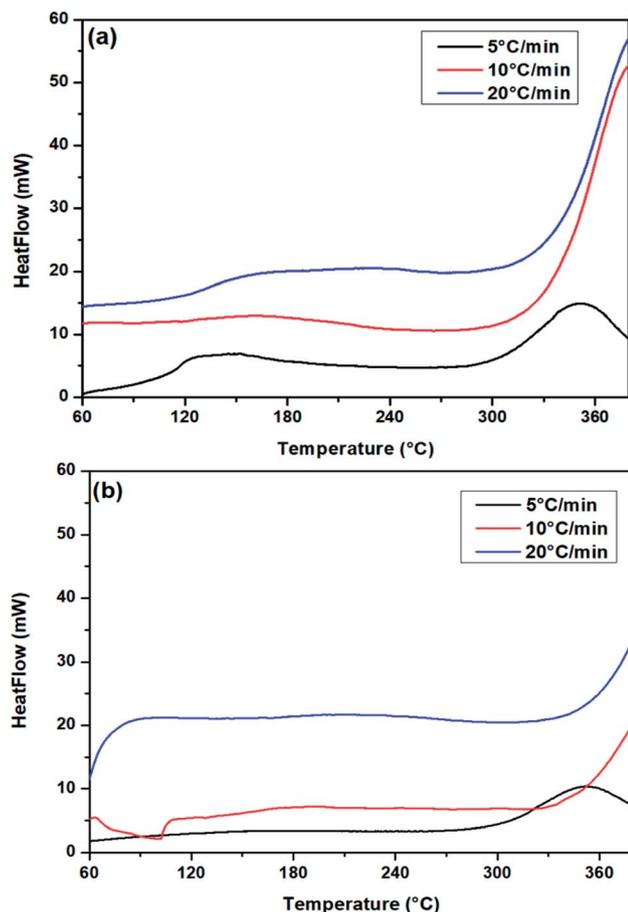
Fig. 8 DSC curves of PUR (HTPB/IPDI) with (a) no catalyst and (b) PS-Im-FeCl<sub>3</sub> at different heating rate.
