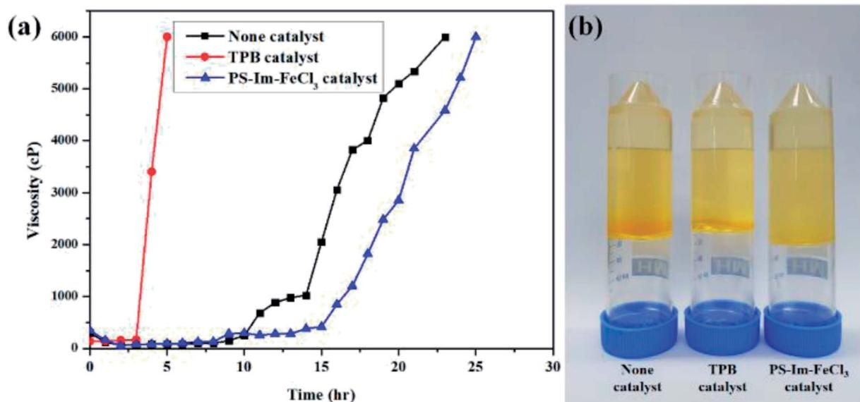
Fig. 7 (a) Viscosity data for polyurethane curing at 60 °C using TPB, no catalyst, and PS-Im-FeCl<sub>3</sub>. (b) Digital images of PU after polymerization.
