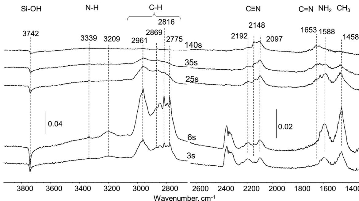
Fig. 3 Difference *in situ* FTIR spectra of Pt/SiO<sub>2</sub> sample exposed to UDMH pulse in He flow at 260 °C.
