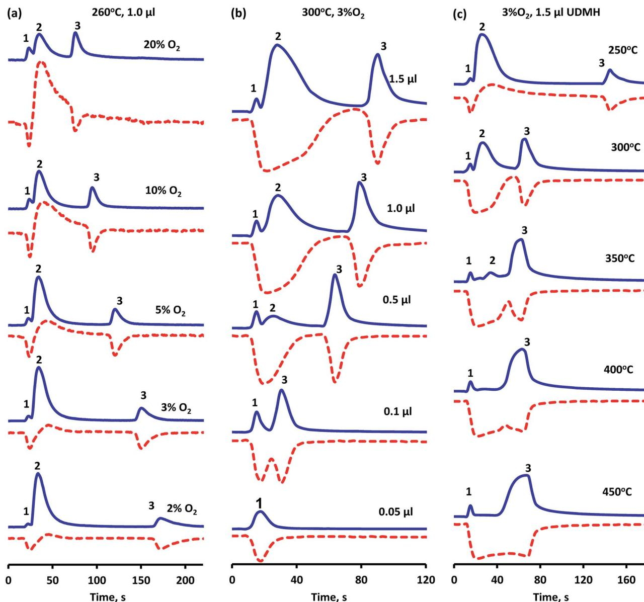
Fig. 7  $\text{CO}_2$  evolution (—  $m/z = 44$ ) and oxygen consumption (---  $m/z = 32$ ) vs. time with variation of reaction conditions: (a) oxygen content in He flow; (b) UDMH pulse volume, (c) reaction temperature.
