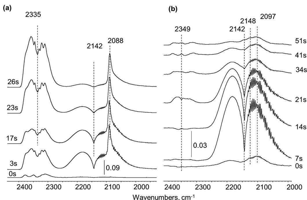
Fig. 4 CO pulsing over  $\text{Pt}/\text{SiO}_2$  sample: (a) fresh, (b) pre-covered with residues from UDMH conversion.
