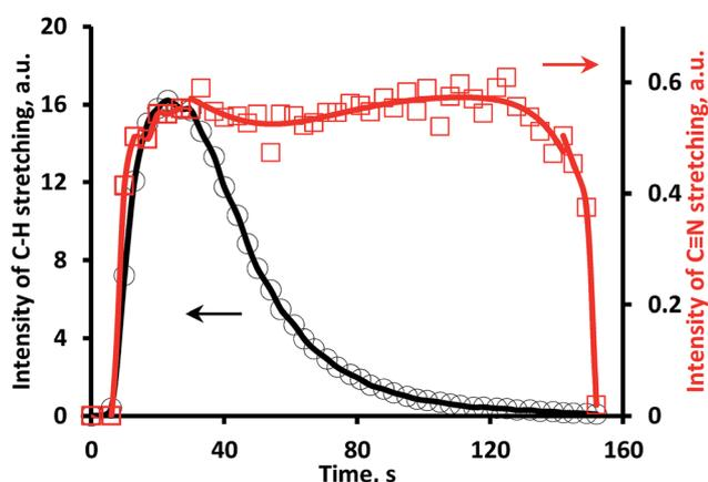
Fig. 6 Total area of all bands in C–H and  $C\equiv N$  stretching regions vs. time after UDMH pulse in 3%O<sub>2</sub>/He flow.
