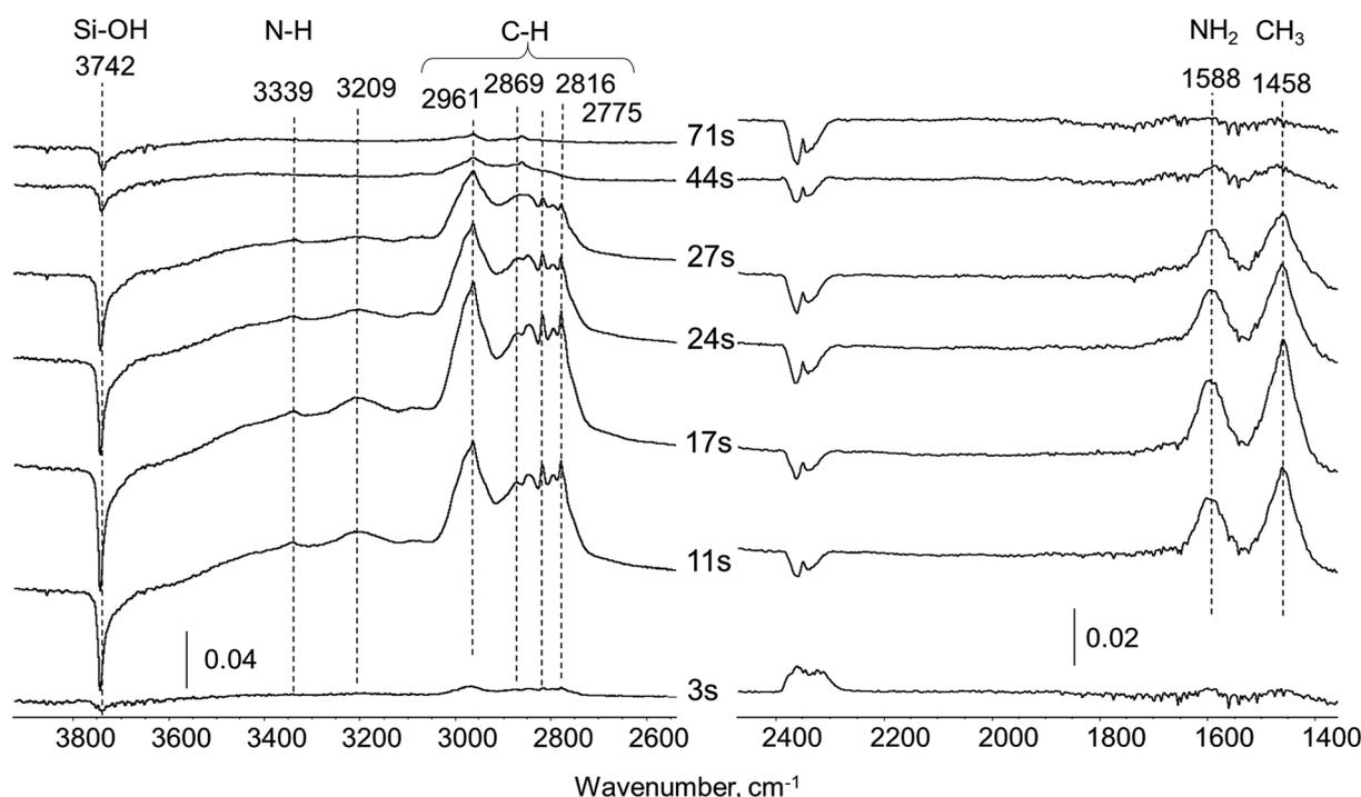
Fig. 2 Difference *in situ* FTIR spectra of silica carrier exposed to UDMH pulse (0.5  $\mu$ l) in 20 ml min<sup>-1</sup> He flow at 260 °C.
