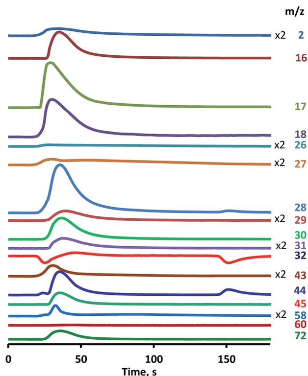
Fig. 1 UDMH conversion over Pt/SiO<sub>2</sub> catalyst. O<sub>2</sub> (3%) He flow, single UDMH pulse, 260 °C, mass-spectrometric detection of reaction products.
