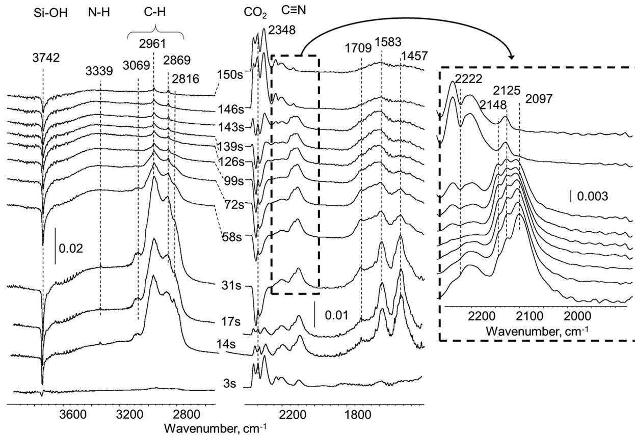
Fig. 5 *In situ* FTIR spectra of Pt/SiO<sub>2</sub> sample exposed to UDMH pulse in 3%O<sub>2</sub>/He flow at 260 °C.
