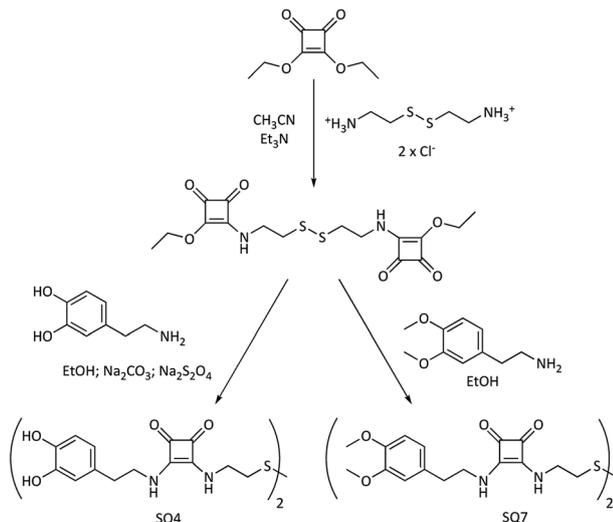
Fig. 3 Synthesis of bis-di-squaramide-dopamine-disulfide and bis-di-squaramide-3,4-dopamine-disulfide receptors.
