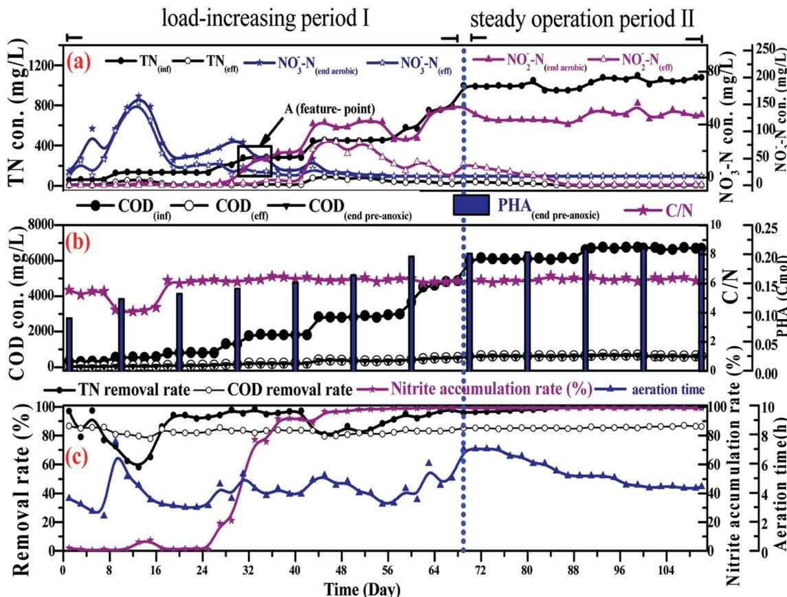
Fig. 4 The treatment performance of the SBBR over the whole operation period.
