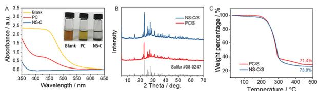
Fig. 3 Lithium polysulfides adsorption test. (A) UV-Vis spectra of bare  $\text{Li}_2\text{S}_6$  solution and after being immersed with PC and NS-C carbons, respectively; the inset picture shows the color change after lithium polysulfides adsorption test, and the blank  $\text{Li}_2\text{S}_6$  solution was used as a control. (B) XRD pattern after sulfur mixed and (C) thermogravimetric curves of sulfur deposited materials of PC/S and NS-C/S.
