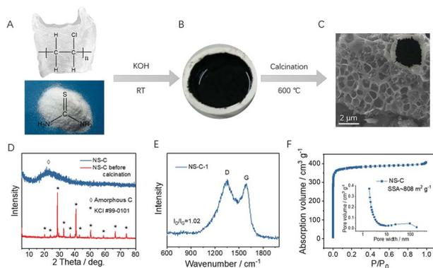
Fig. 1 Fabrication process, morphology characterization and the physical properties of the porous structure materials (NS-C). (A) Raw materials. (B) End-product of the NS-C sample. (C) SEM image of NS-C shows a cellular structure. (D) XRD pattern. (E) Raman spectra and (F) pore size distribution of the NS-C samples.
