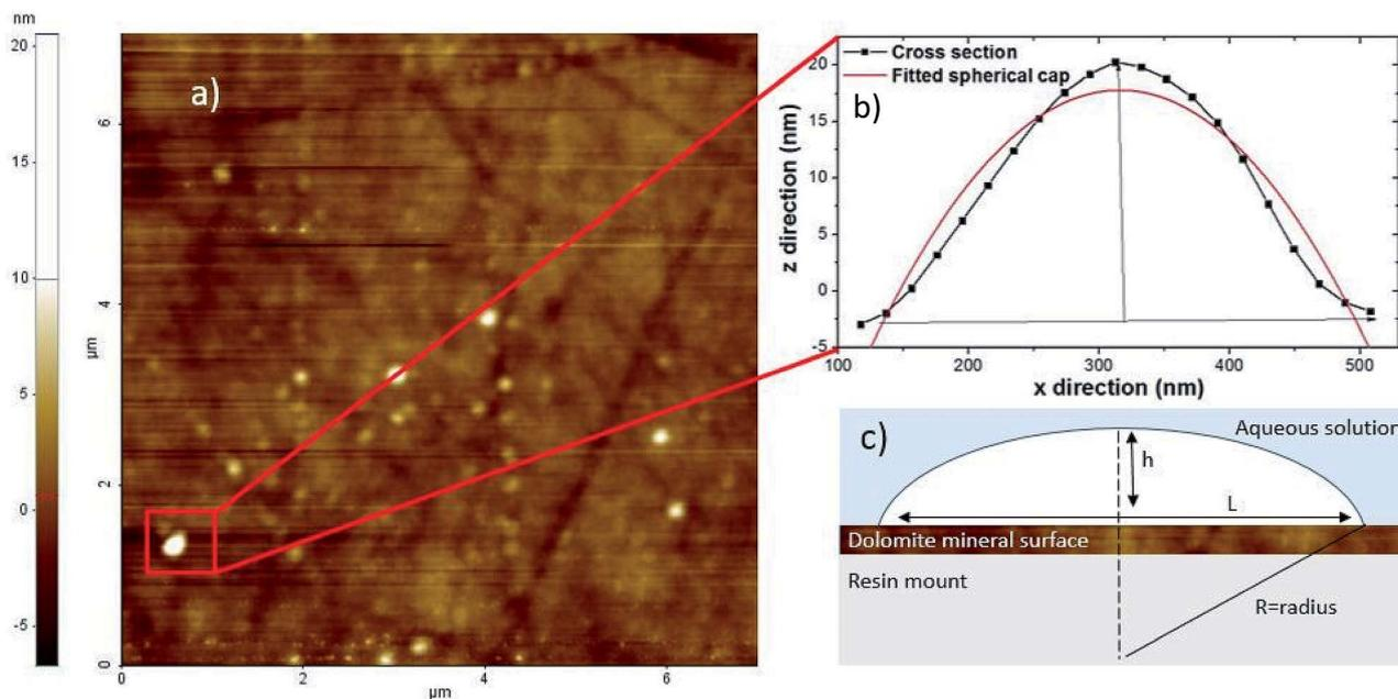
Fig. 2 (a)  $8\ \mu\text{m} \times 8\ \mu\text{m}$  non contact atomic force microscopy (AFM) image of surface nanobubbles on the carbonate mineral dolomite (b) cross section of nanobubble height and width extracted from the non contact AFM image (c) diagram of height ( $h$ ), length ( $L$ ) and radius ( $R$ ) with contact angle ( $\theta$ ) of the nanobubble. Diagram (c) after Lohse and Zhang.<sup>14</sup>
