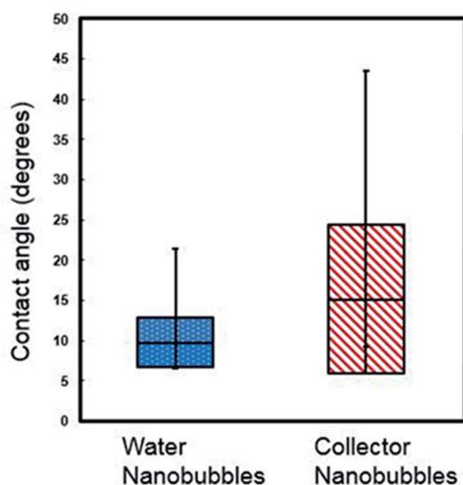
Fig. 3 Box and whisker plot of contact angles of nanobubbles under collector and DI water conditions (the data was selected using fitting of a spherical cap model after Lohse and Zhang.<sup>14</sup>
