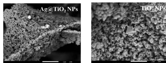
Fig. 2 SEM micrographs of  $\text{Ag@TiO}_2$  and  $\text{TiO}_2$  particles.
