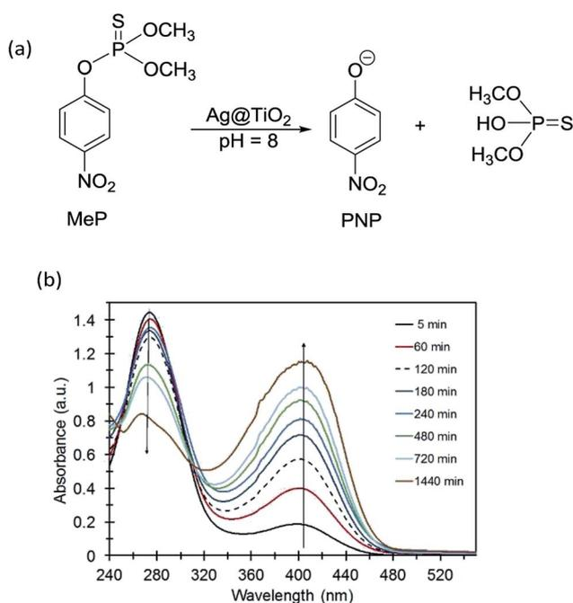
Fig. 3 (a) Hydrolysis of methyl parathion using core-shell Ag@TiO<sub>2</sub>. (b) UV-Vis spectra for methyl parathion + Ag@TiO<sub>2</sub> vs. time.
