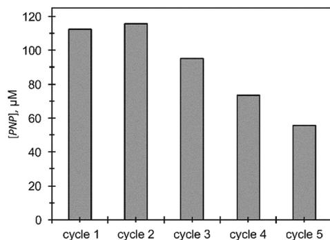
Fig. 9 Reusability test for Ag@TiO<sub>2</sub> in MeP hydrolysis.
