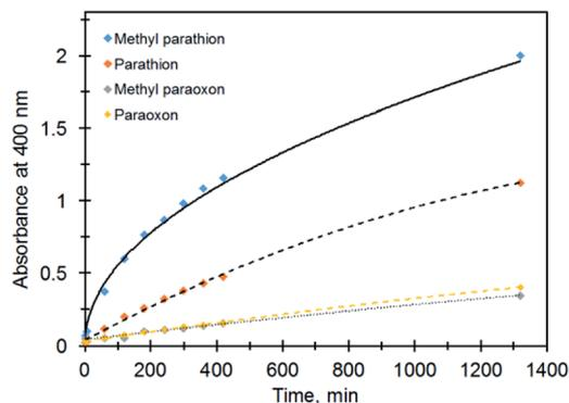
Fig. 7 Profiles of absorbance (PNP, 400 nm) vs. time for different organophosphates in the presence of Ag@TiO<sub>2</sub>.
