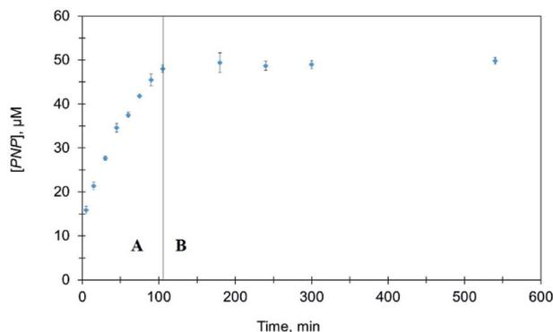
Fig. 8 Comparison of PNP formation in the presence and absence of Ag@TiO<sub>2</sub>. (A) Before removal of Ag@TiO<sub>2</sub> (B) after removal of Ag@TiO<sub>2</sub>.
