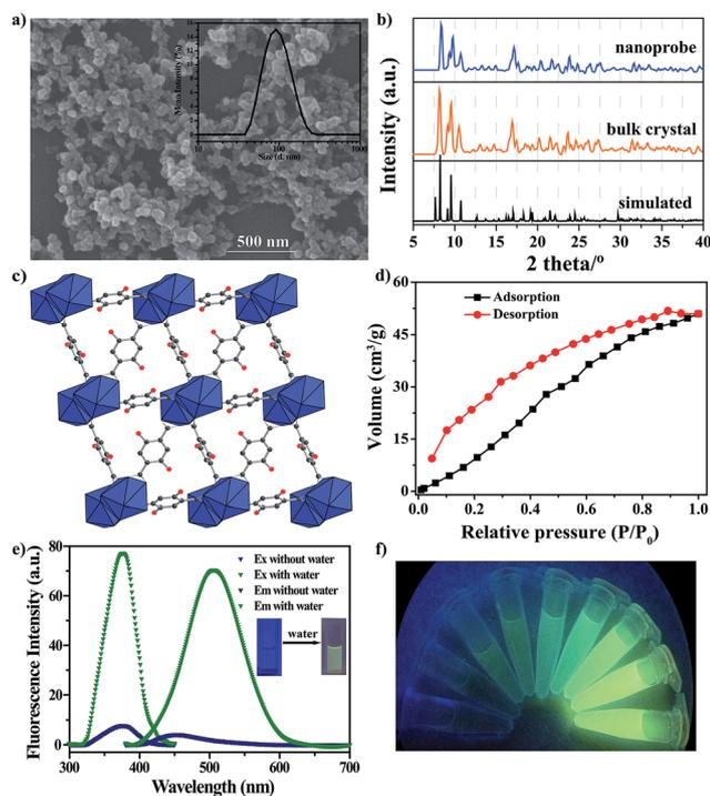
Fig. 1 (a) SEM image. The inset shows the DLS analysis. (b) XRD patterns. (c) The framework. (d)  $CO_2$  adsorption/desorption isotherms obtained for the nanoprobe. (e) Fluorescence excitation (Ex) and emission (Em) spectra of the nanoprobe dispersion in dry MeCN without and with water. (f) Visible color changes of the nanoprobe in the presence of successive aliquots of water when irradiated with UV light of 365 nm. The water content was 0, 0.05, 0.5, 1, 2, 3, 4, 5 and 6% v/v.
