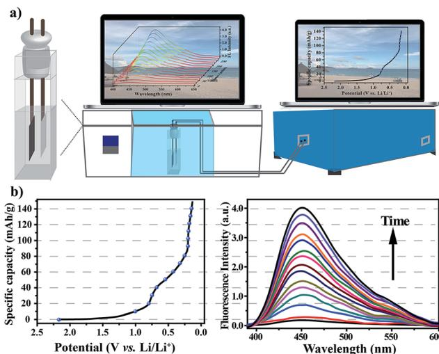
Fig. 5 (a) A schematic diagram of the home-made *in situ* cell and measurement system. (b) Changes in the fluorescence spectra of the electrolyte with the nanoprobe as an electrolyte additive during the first discharge process.
