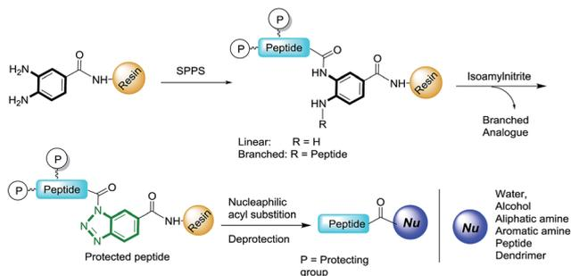
Fig. 1 Representative scheme for the on-resin C-terminal modification of peptide analogues. A linear analogue has the Dbz moiety on one peptide. Branched analogues have two peptides attached to one Dbz moiety.
