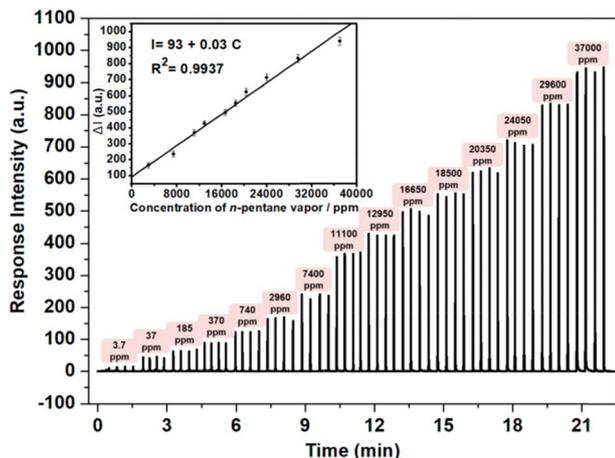
Fig. 6 The net responses of different concentrations (from 3.7 ppm to  $3.7 \times 10^4$  ppm) of *n*-pentane to the fluorescence emission of S7 ( $\lambda_{\text{ex}}/\lambda_{\text{em}} = 460 \text{ nm}/678 \text{ nm}$ ) at 293 K, the measurements of which were taken on the home-made sensing platform. Inset: a plot of the differences in the response intensities against the concentrations of *n*-pentane.
