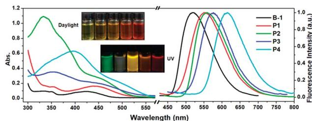
Fig. 1 UV-Vis absorption and normalized fluorescence emission spectra ( $\lambda_{\text{ex}} = 405$  nm) of monomer B-1, polymers P1–P4 in  $\text{CHCl}_3$  at  $0.02 \text{ mg mL}^{-1}$ . Inset: photos of the corresponding solutions under daylight and UV light (365 nm).
