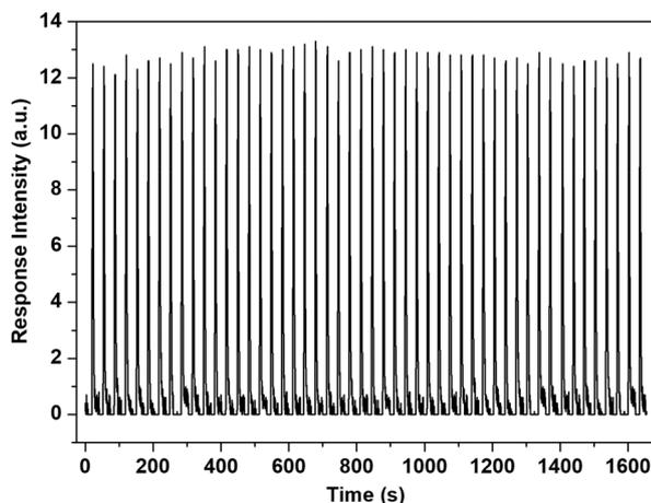
Fig. 7 Results from 50 repeats of a reusability test for S7 towards the *n*-pentane vapor measured on the home-made sensing platform at 293 K. Saturated *n*-pentane vapor was used as the sample analyte and the vapor was sampled (3 mL for each measurement) using the stationary gas supply system (Fig. S7<sup>†</sup>).
