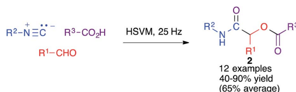
Scheme 2 The mechanochemical Passerini reaction.
