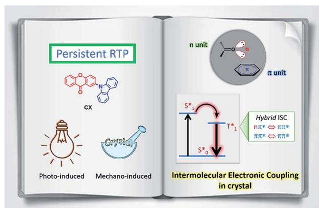
Fig. 1 Schematic diagram of the intermolecular electronic coupling in the crystalline state for persistent RTP: (left) chemical structure of the compound CX, (above right) intermolecular n- and  $\pi$ -units stacked in the crystal, and (below right) hybrid intersystem crossing formation.  $S_0^*$  = the ground state,  $S_1^*$  = the lowest singlet excited state, and  $T_1^*$  = the lowest triplet excited state. All these states refer to the proposed intermolecular electronically coupled states.
