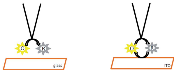
Scheme 2 Role of the electrofluorochromic mediator in the feedback mode on insulating (left) and conducting (right) substrates.
