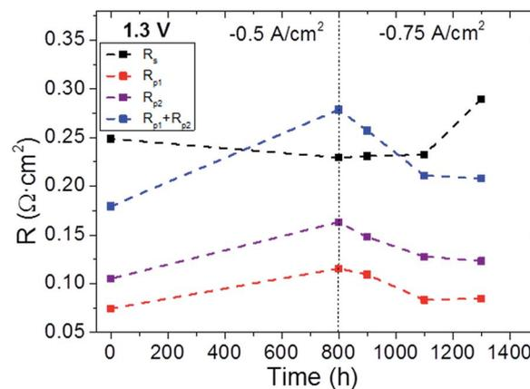
Fig. 6 Evolution of serial ( $R_s$ ) and polarization ( $R_{p1}$ ,  $R_{p2}$ ,  $R_{p1} + R_{p2}$ ) resistances with time recorded at 1.3 V. Dashed lines come from interpolation and are only included as guides for the eye.
