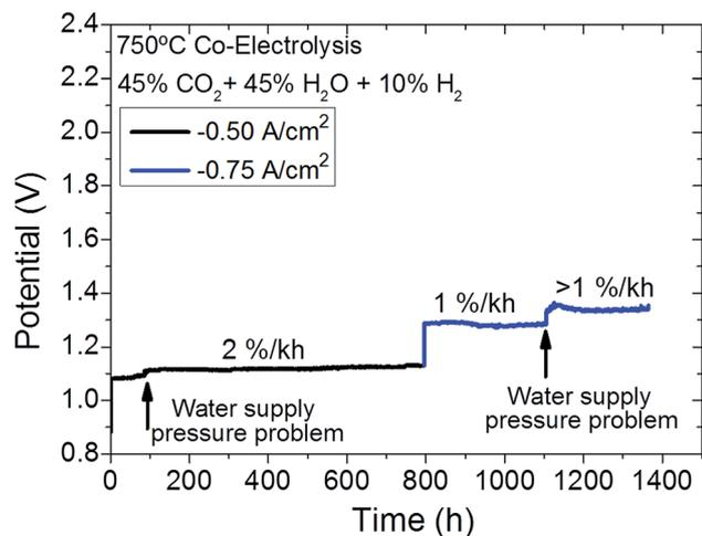
Fig. 4 Long term testing of mesoporous oxygen electrode when 0.5 and 0.75 A cm<sup>-2</sup> current densities are injected, operating under co-electrolysis 45% H<sub>2</sub>O + 45% CO<sub>2</sub> + 10% H<sub>2</sub> and synthetic air gas atmospheres at fuel and oxygen electrodes, respectively.
