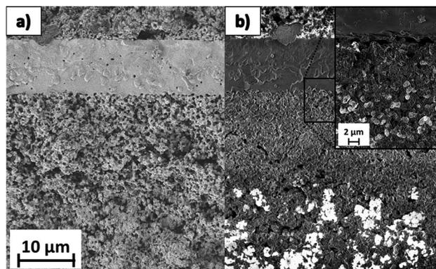
Fig. 8 Cross section of the interface between the fuel electrode and the electrolyte of the cell after 1400 h of operation taken using (a) secondary electron (SE2) and (b) Inlens SEM detectors.
