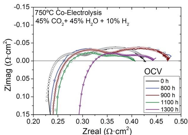
Fig. 5 Nyquist plot of the EIS as obtained at co-electrolysis and synthetic air gas composition atmospheres for a cell operating at 750 °C at different times at OCV. Each fitting, based on the equivalent circuit  $LR_s(R_{p1}Q_1)(R_{p2}Q_2)$ , is indicated by a continuous line.
