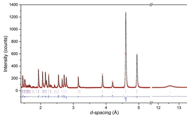
Fig. 3 Rietveld refinement of high resolution neutron diffraction patterns of  $\text{MnFe}_3\text{O}_5$  obtained at 5 K, with upper tick marks indicating nuclear peaks and lower presenting magnetic reflections. ( $R_{wp} = 12.9\%$  and  $R_p = 12.6\%$ ).
