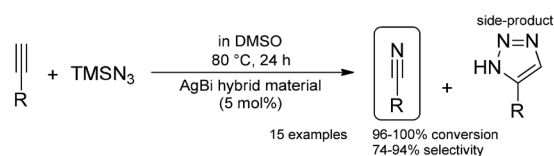
Scheme 27 Heterogeneous AgBi hybrid material-catalysed direct alkyne nitrogeneration. 120
