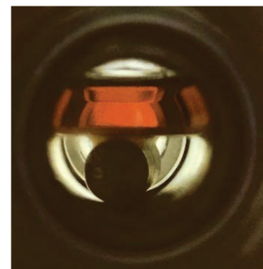
Fig. 2 Observed catalyst partitioning for 2 in a typical experiment prior to addition of reaction gases. (Top: orange n -decane phase containing the catalyst; bottom: colorless MeOH phase with 1,2-dimethyl-imidazole (1,2-DMI).
