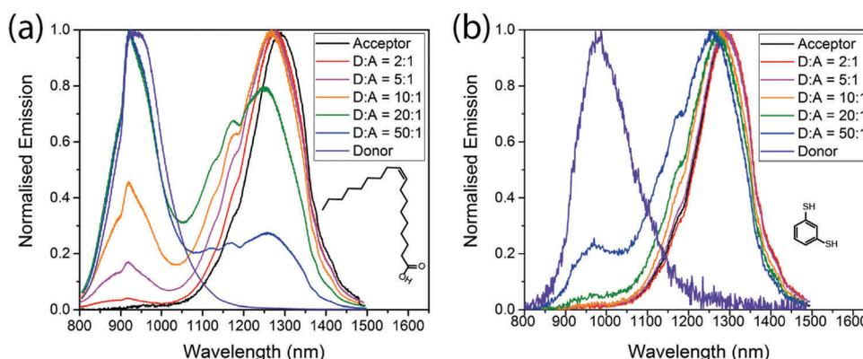
Fig. 3 Emission spectra of different donor : acceptor blends, with oleic acid ligands (a) and benzenedithiol ligands (b) excited at 405 nm.
