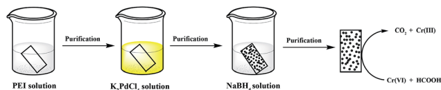
Scheme 1 Schematic illustration of the immobilization of Pd NPs onto filter paper for catalytic applications.
