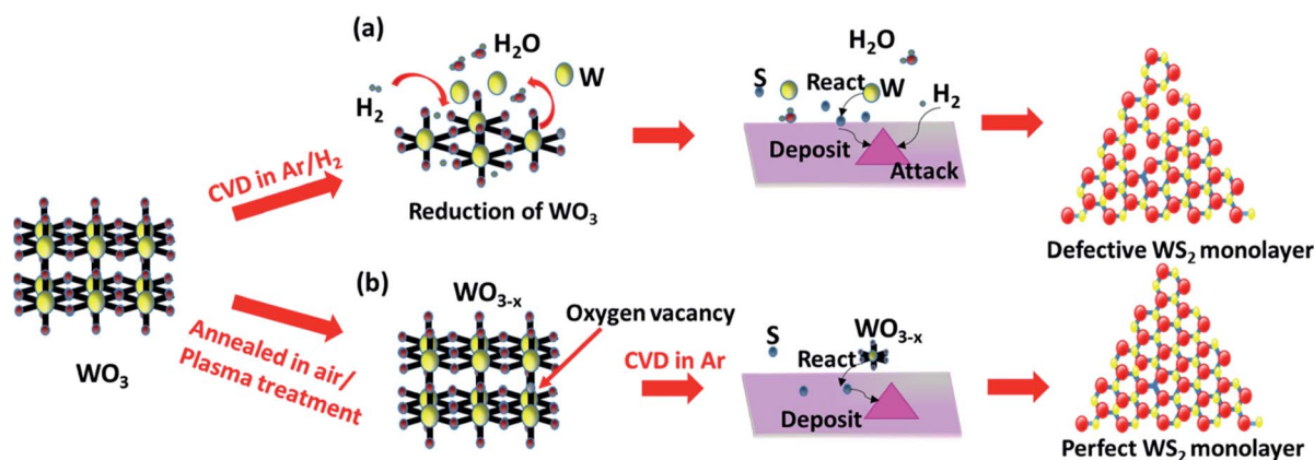
Fig. 1 Reaction mechanism for CVD growth of (a) the commercial precursor in an Ar/H 2 atmosphere; (b) pretreated precursors in an Ar only atmosphere.
