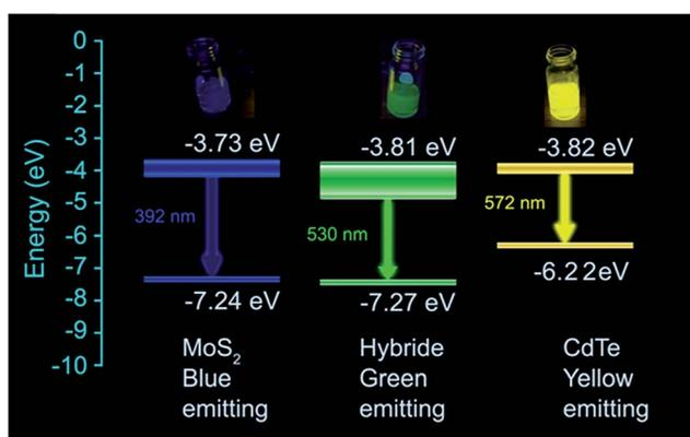
Scheme 1 Band diagram of MoS<sub>2</sub> QDs, capped yellow emissive CdTe QDs and the formed hybrid structure having 1 : 1 volumetric ratio of individual QDs.
