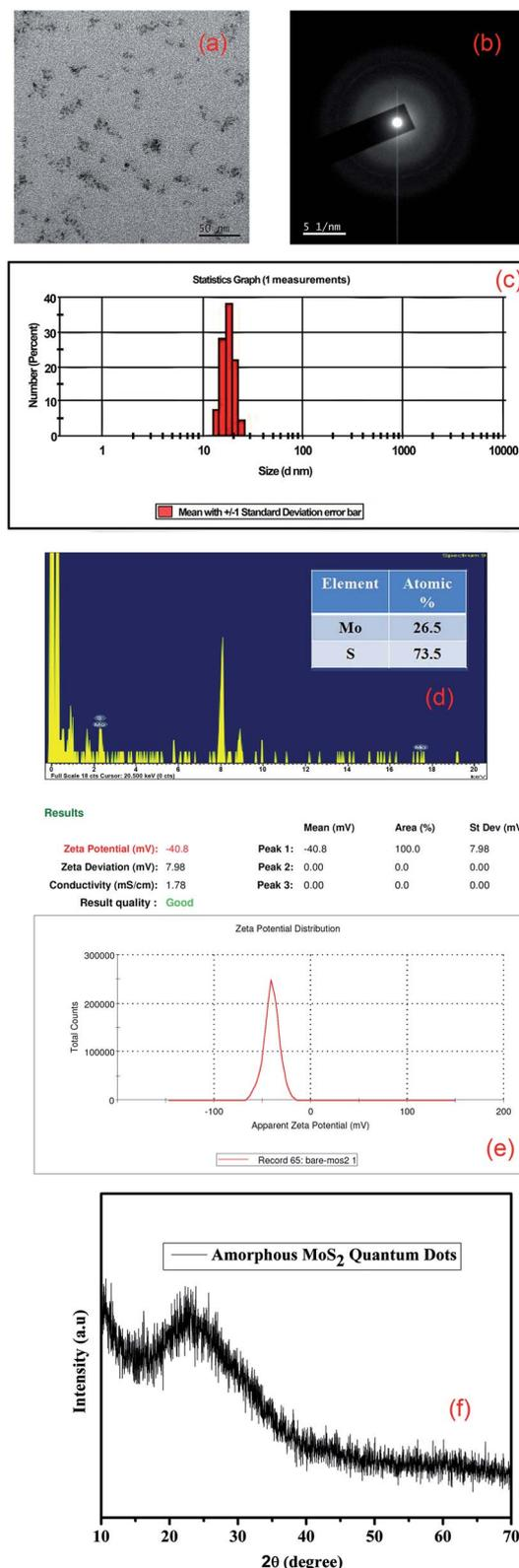
Fig. 1 (a) TEM image of the as-synthesized MoS<sub>2</sub> QDs; (b) SAED pattern of the as-synthesized amorphous MoS<sub>2</sub> QDs; (c) particle size distribution of MoS<sub>2</sub> QDs from DLS measurements; (d) EDX analysis of sulfur-rich MoS<sub>2</sub> QDs; (e) zeta potential of sulfur rich MoS<sub>2</sub> QDs; (f) XRD pattern of the as-synthesized amorphous MoS<sub>2</sub> QDs.
