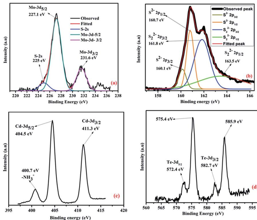
Fig. 5 (a) XPS spectra of S-2s, Mo(IV)-3d<sub>5/2</sub> and 3d<sub>3/2</sub> in hybrid QDs; (b) deconvoluted XPS spectra of S<sup>2-</sup>-2p<sub>3/2</sub> and 2p<sub>1/2</sub> and S<sub>2</sub><sup>2-</sup>-2p<sub>3/2</sub> and 2p<sub>1/2</sub> in hybrid QDs; (c) XPS spectra of N-1s in -NH<sub>3</sub><sup>+</sup> attached with the CdTe surface and Cd-3d<sub>5/2</sub> and Cd-3d<sub>3/2</sub> of hybrid QDs; (d) XPS spectra of Te<sup>2-</sup>-3d<sub>5/2</sub> and 3d<sub>3/2</sub> in hybrid QDs.
