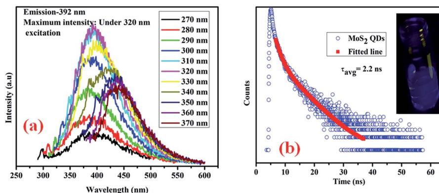
Fig. 6 (a) Excitation dependent photoluminescence emission spectra of bare MoS<sub>2</sub> QDs; (b) time-correlated single photon counting (TCSPC) of the as-synthesized MoS<sub>2</sub> QDs and an actual photograph of the emission of bare MoS<sub>2</sub> QDs under UV light (inset).
