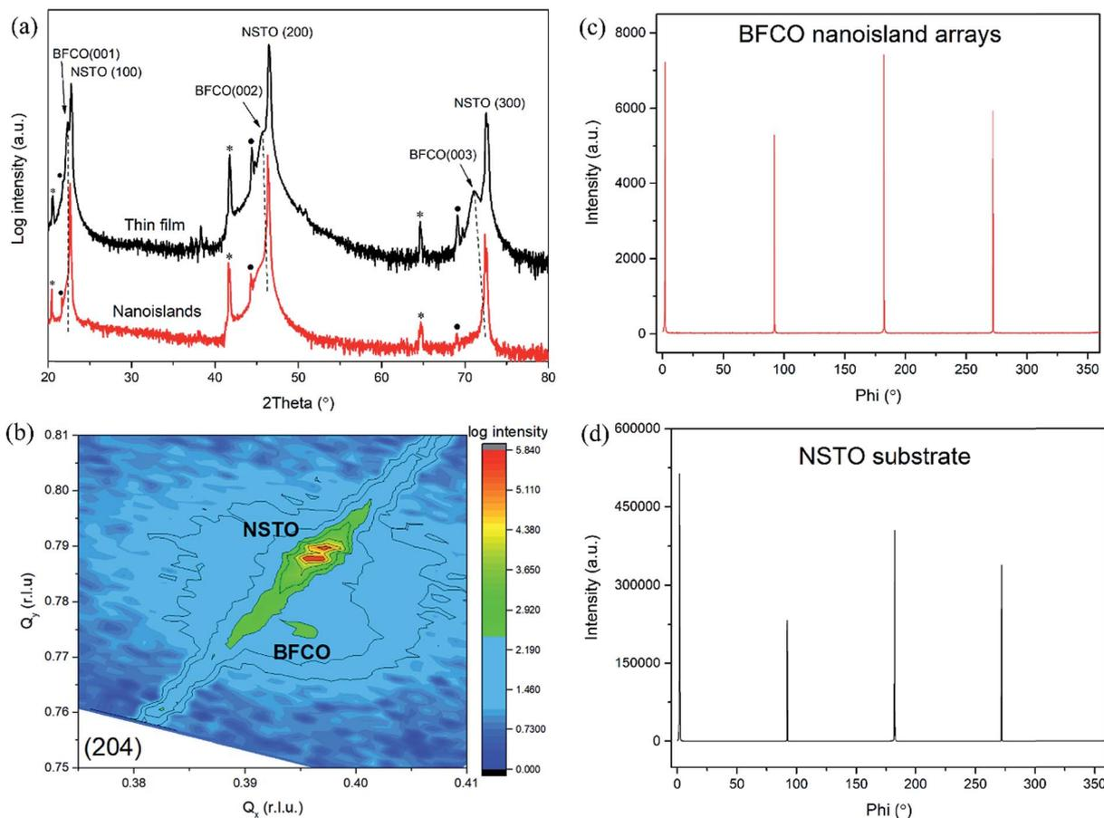
Fig. 3 XRD patterns of the BFCO nanoisland arrays grown on the NSTO substrate: (a)  $\theta$ - $2\theta$  scan (the BFCO thin film deposited under the same deposition conditions was also analyzed for comparison). The stars correspond to the (00l)  $K_{\beta}$  line, and the points indicate tungsten contamination of the X-ray cathode tube. (b) RSM around the (204) plane of the NSTO substrate; Phi-scan around the (110) plane for (c) BFCO nanoisland arrays and (d) NSTO substrate.
