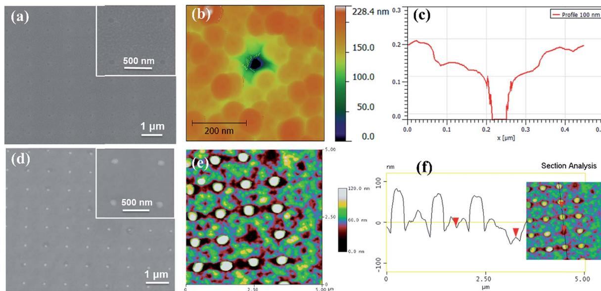
Fig. 2 (a) SEM micrograph (inset shows the magnified view), (b) AFM topography image, and (c) depth profile of the SiO<sub>2</sub> hard mask. (d) SEM micrograph (inset shows the magnified view), (e) AFM topography image, and (f) depth profile of the BFCO nanoisland arrays after removing the SiO<sub>2</sub> mask.
