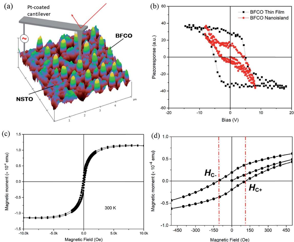
Fig. 4 (a) Schematic illustration of PFM analysis for BFCO nanoisland arrays/NSTO with a 3D-AFM topography image of  $5 \times 5 \mu\text{m}^2$  area. (b) Local PFM measurements of an individual BFCO nanoisland and the BFCO thin film for comparison. (c) Magnetization hysteresis loop for BFCO nanoisland arrays on NSTO (100) in the field range of 10 kOe at 300 K measured using a SQUID magnetometer. (d) Magnification of the magnetization hysteresis loop in the range of  $\pm 525$  Oe.
